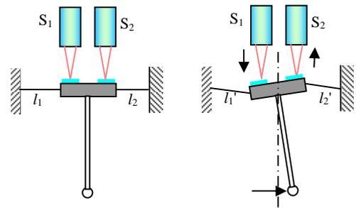
Fig. 11. Structure and motion of a touch probe
