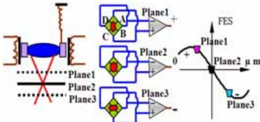
Fig. 3. The variation of spot shape with distance producing a S-curve of FES
