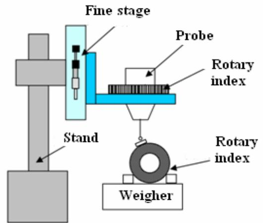
Fig. 13. Setup for probe calibration
