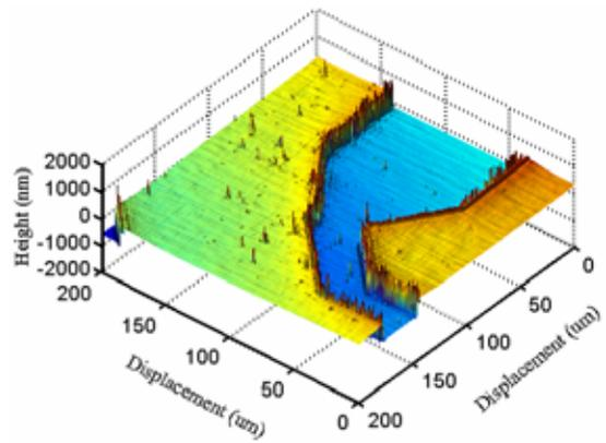
Fig. 5. Measured sample (Nickel on ALGaN)
