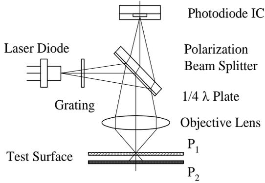
Fig. 2. Principle of focus probe
