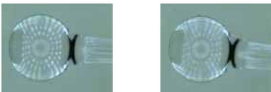
Fig. 10. Fabricated ball tips on a glass fiber
