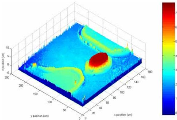
Fig. 9. Measured spacer profile by confocal microscope
