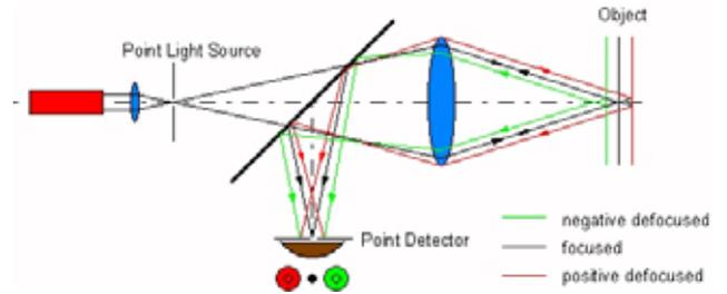
Fig. 6. Laser confocal probe
