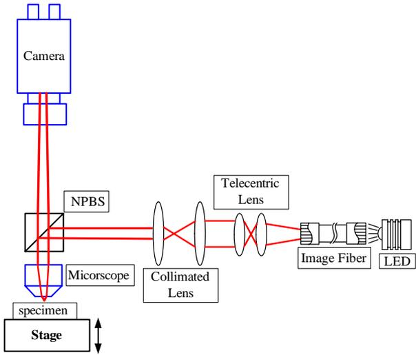
Fig. 7. Image fiber confocal microscope
