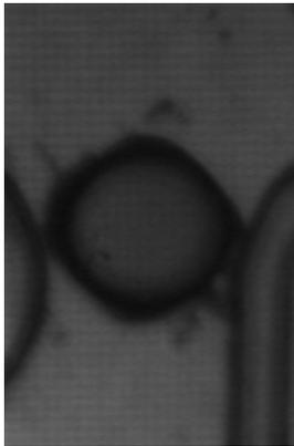
Fig. 8. Image shows focusing on the substrate of LCD spacer
