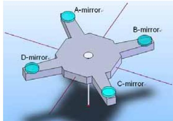
Fig. 12. Mechanism of the contact probe
